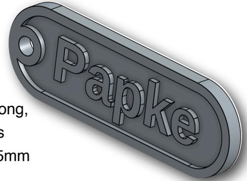
Your name tag should look like the picture to the right. It is 75mm long, 25mm high and 4mm thick. The hole has a diameter of 5mm and is 6mm from the side. The text size is 10-15mm. The “Extrude” is 2.5mm
